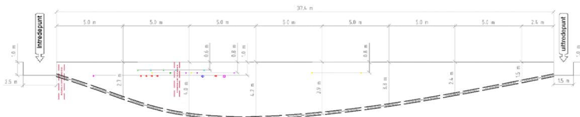
Boring JMS436560 Mantelbuis HDPE Ø125mm
